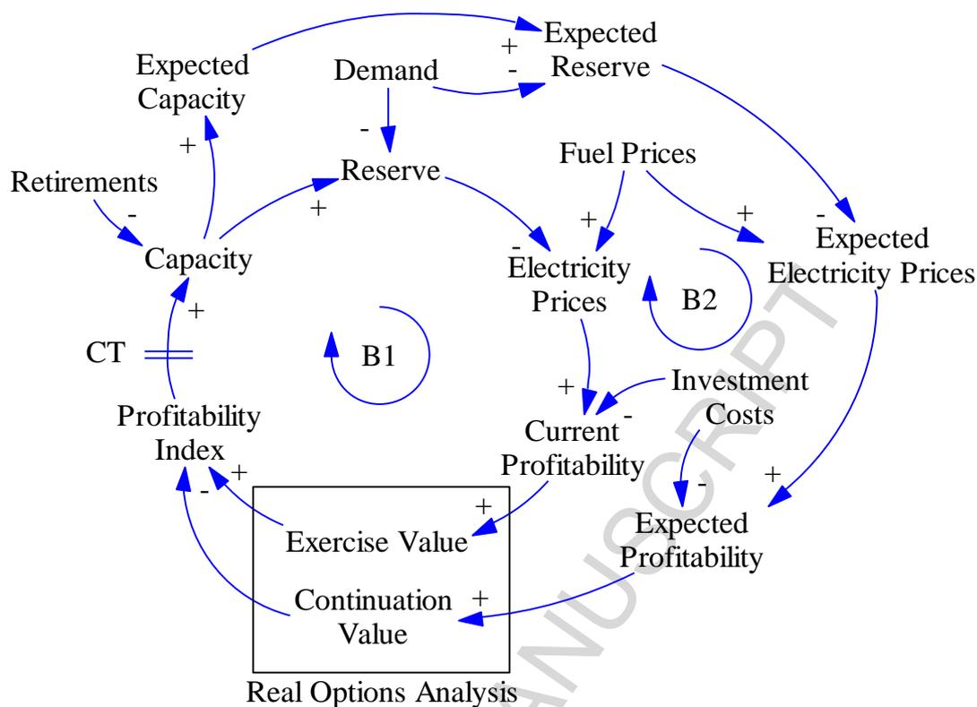
Fig. 1: Causal-loop Diagram of the long-term development of electricity markets under the proposed decision-making framework.
