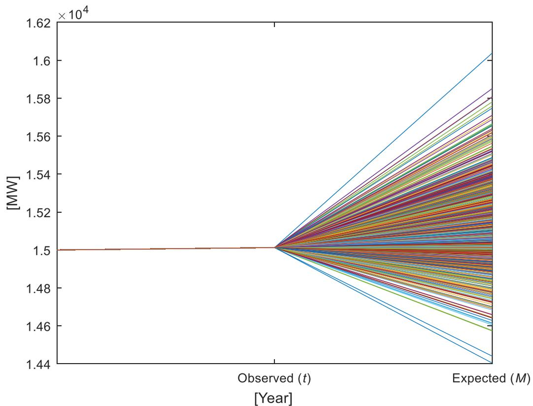
Fig. 4: Simulation of the observed and expected maximum demand at time  $t$  after the beginning of simulations.
