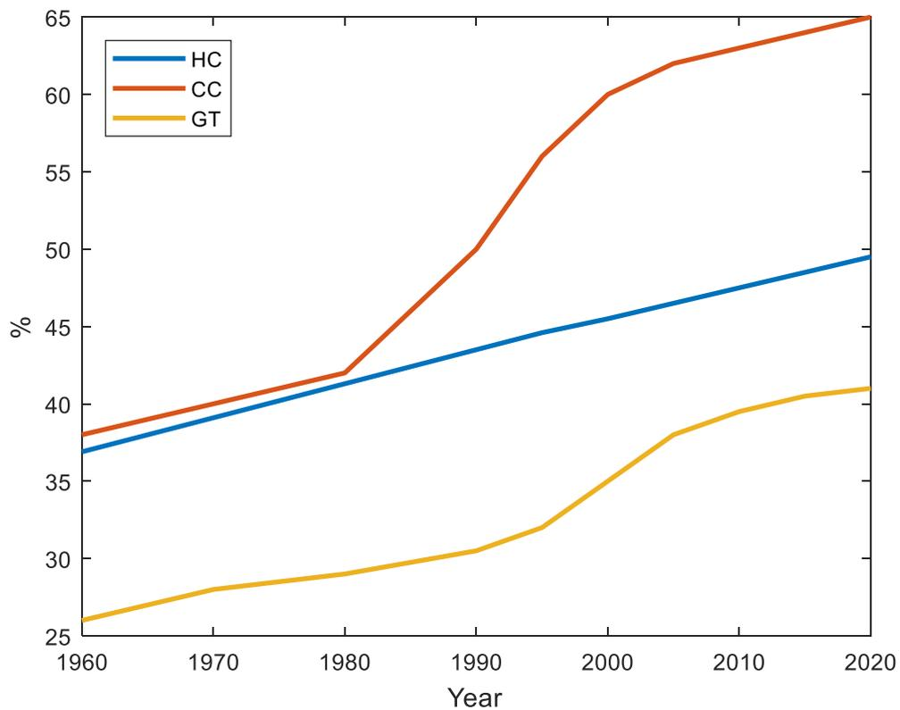
Fig. 2: Estimation of evolution of thermal efficiencies for the technologies in the test generation system.
