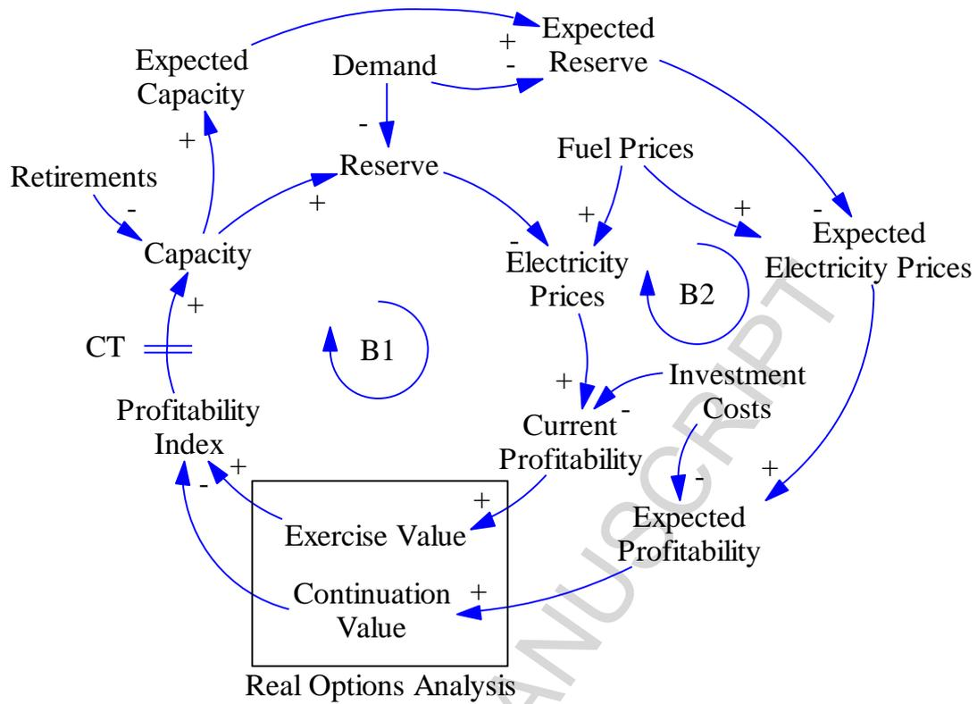
Fig. 1: Causal-loop Diagram of the long-term development of electricity markets under the proposed decision-making framework.
